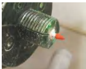
▲ Pic.12 The nose is a 6mm piece of maple with a 4mm peg. Stain orange using spirit stain and glue it into the head
